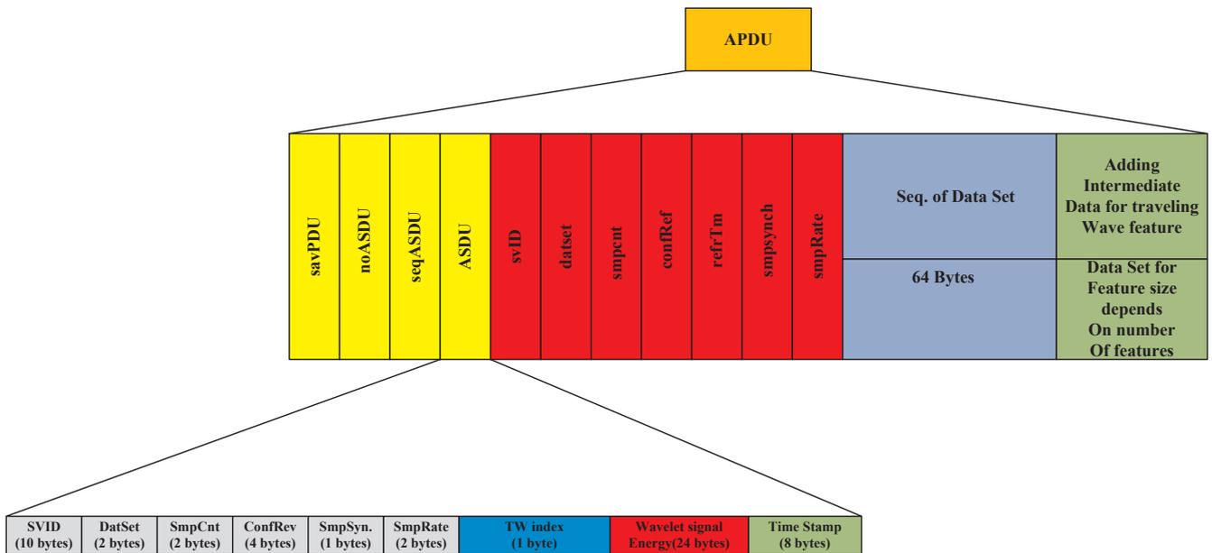
Fig. 10. Modified IEC 61850-9-2 SV message format with additional information added to ASDU.
