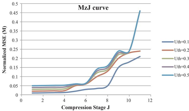
Fig. 5. Relation between mean square error, threshold level, and compression stage.
