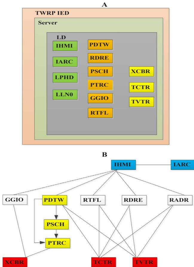
Fig. 11. A – TWRP IED model and B – Decomposition of TWRP functions.
