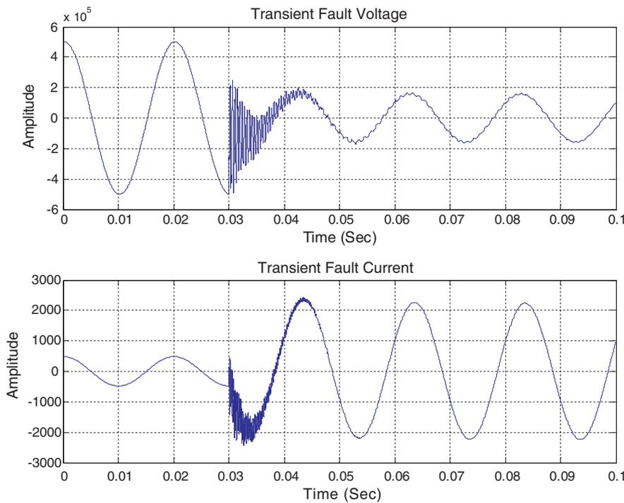
Fig. 7. Travelling wave fault voltage and current signal between phase and ground.
