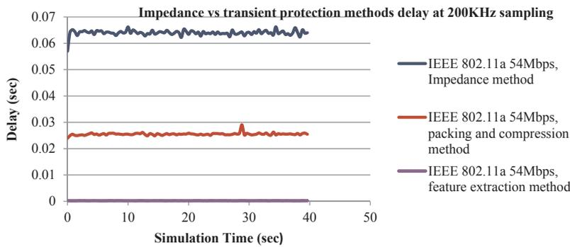
Fig. 12. ETE delay comparison of impedance method Ref. [17] vs our proposed packing & compressing and feature extraction methods.
