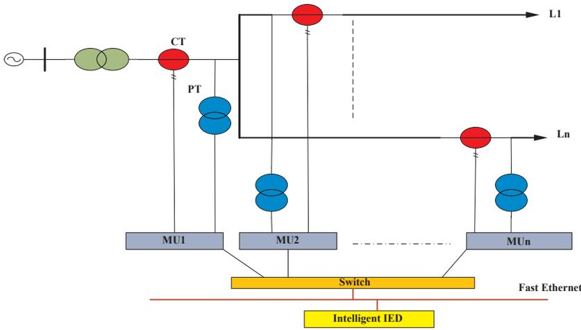
Fig. 2. Multiple MUs network communication of process level based on IEC 61850.
