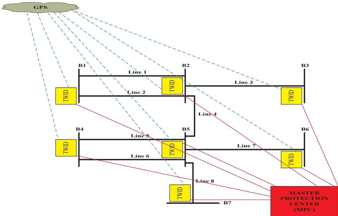
Fig. 1. Proposed WAP based on travelling wave.
