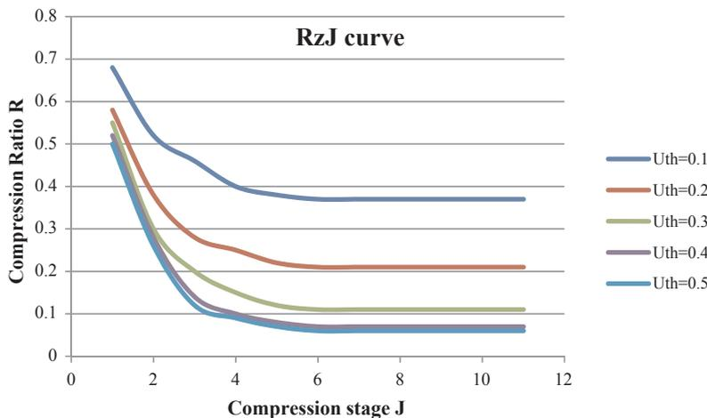
Fig. 6. Relation between compression ratio, threshold level, and compression stage.
