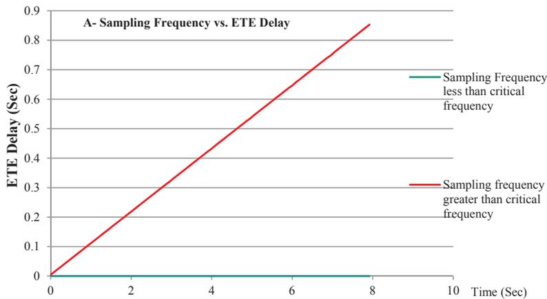
Fig. 3. A – Performance of SAV message ETE delay below and above the critical frequency, B – Relation between sampling frequency and number of MUs at power frequency protection, and C – Relation between sampling frequency and number of MUs based on the travelling wave technique.
